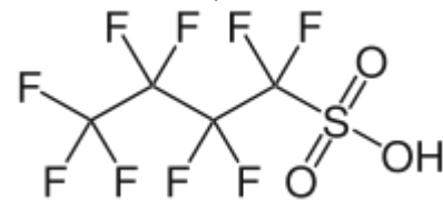
Figure 2 Molecular structure of perfluorooctane sulfonic acid (PFOS).
