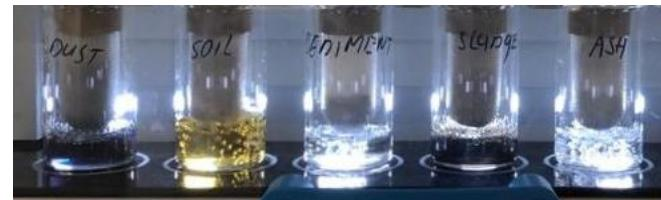
Figure 2 Extraction of the samples according the Randall and Twisselman principle on a SER-158
