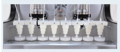
This poster discusses the extraction of **EPA Method 525.2** and **TCLP Semi-volatile Organic Compounds (SVOCs)** using Mini-disks MD-525-30 and MD-BNA-30 with the SPE-03 automated solid phase extraction system.
