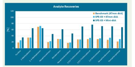
Compared to the 47-mm disk, the improved performance of the Mini-disk is attributed in part to the optimized sorbent proportion, packing distribution and flow design within its housing. The smaller disk area also allows for easier conditioning, drying and elution.
