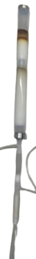
Figure 2 Column set of a 5g dried sewage sludge sample after GO-EHT clean-up from in-house experiments.
